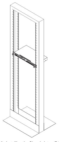
Figure 2-2. Installing the Chassis into a Telco Rack
